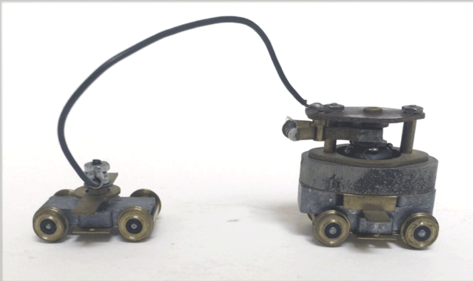
Exhibit A – Bowser 1966 Traction Mechanism with 30” wheels.
